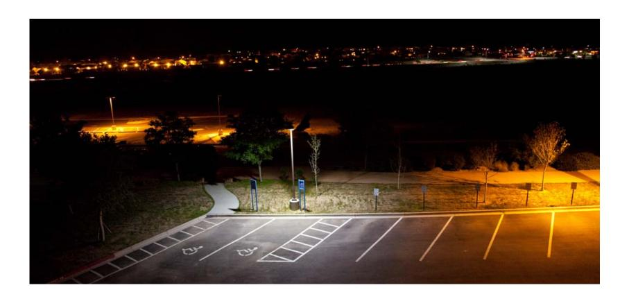
54W LED bulb on the left vs. 250W HPS bulb on the right....
